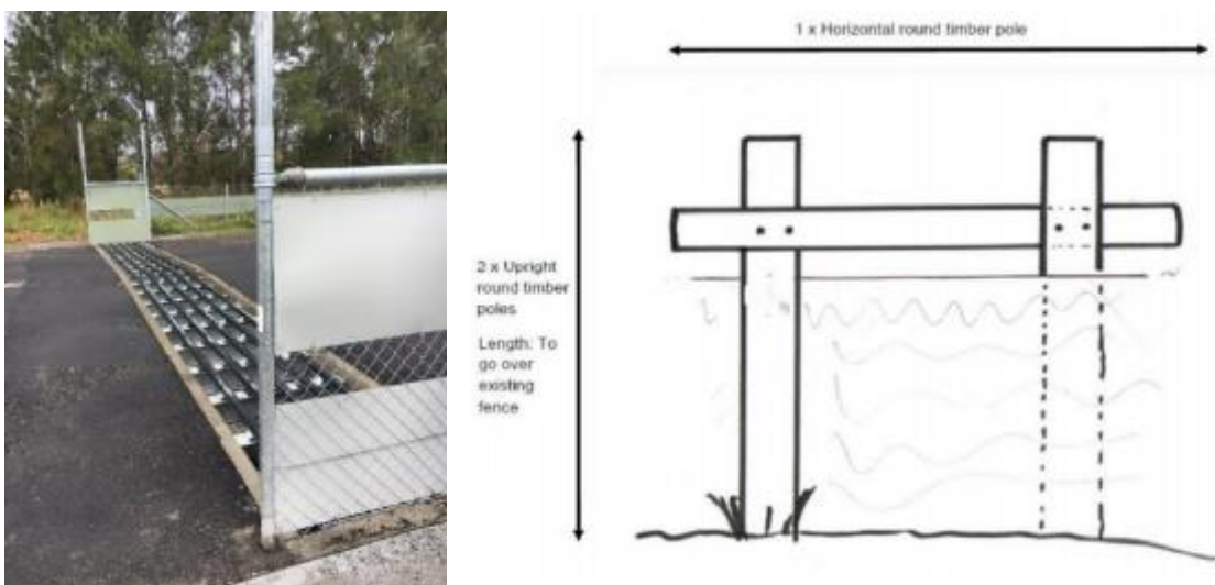
Plate 2-3 Koala structures to be constructed along the perimeter fencing. Left: Koala grids. Right: Koala bridges.
