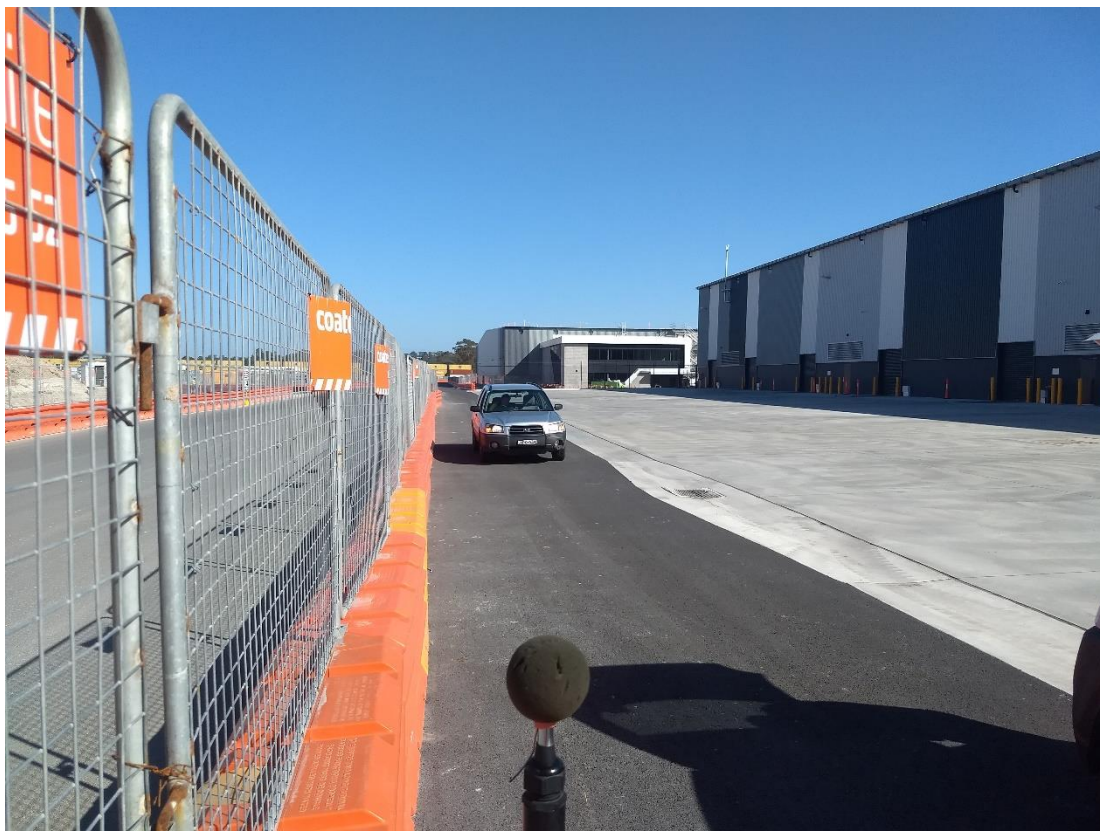
Figure 4 ATS North Unattended Noise Measurement Setup
