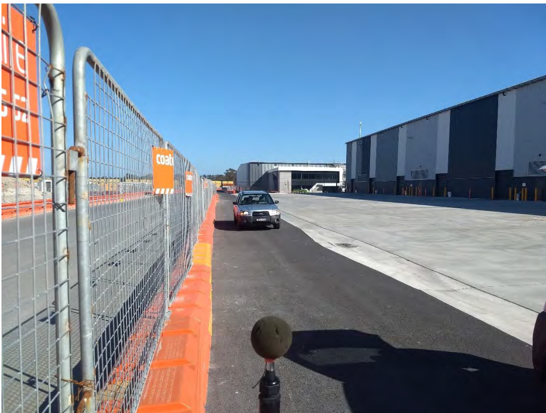
Figure 4 ATS North Unattended Noise Measurement Setup
