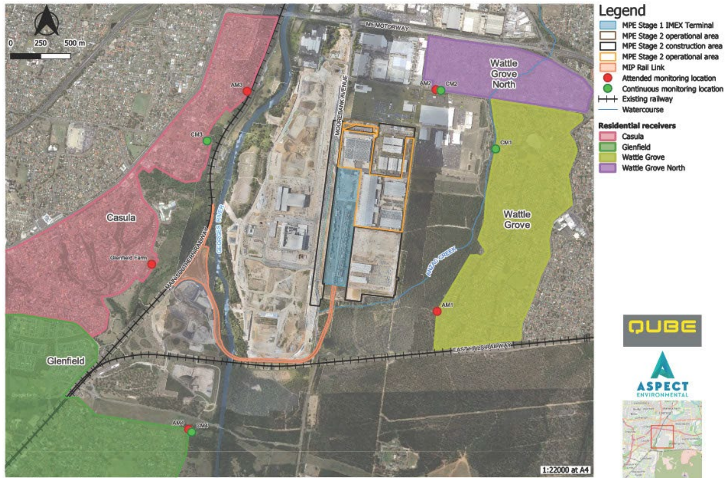
Figure 3-1: Noise Catchment areas and noise monitoring locations
