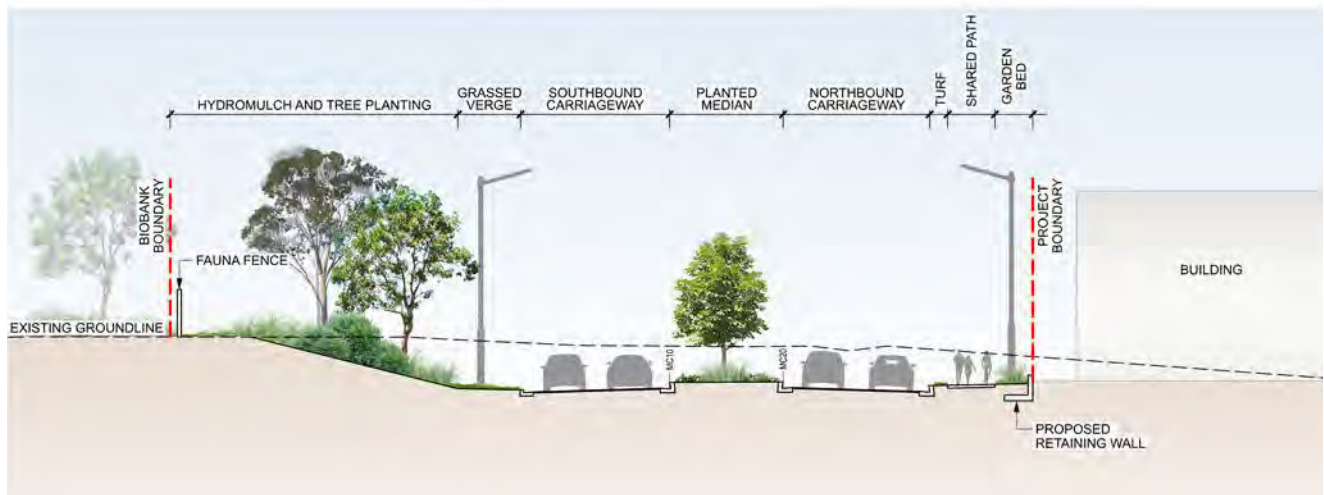
Figure 16. Typical Section B-B at Chainage 1600
