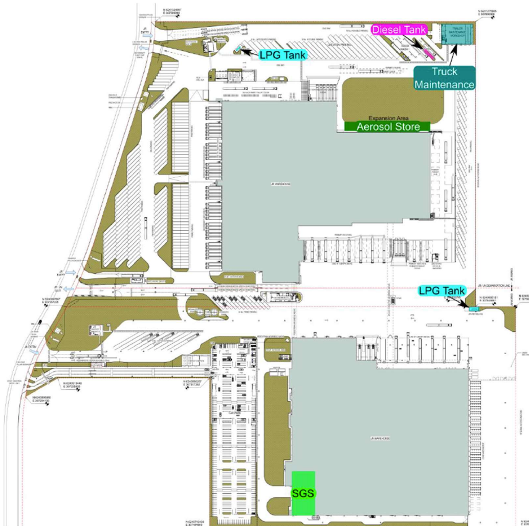
Figure 4-1 MORDC and MONDC Warehouses site layout with dangerous goods storage locations (Final Hazard Analysis, Moorebank Logistics Park, Riskcon Engineering, 30 August 2024)
