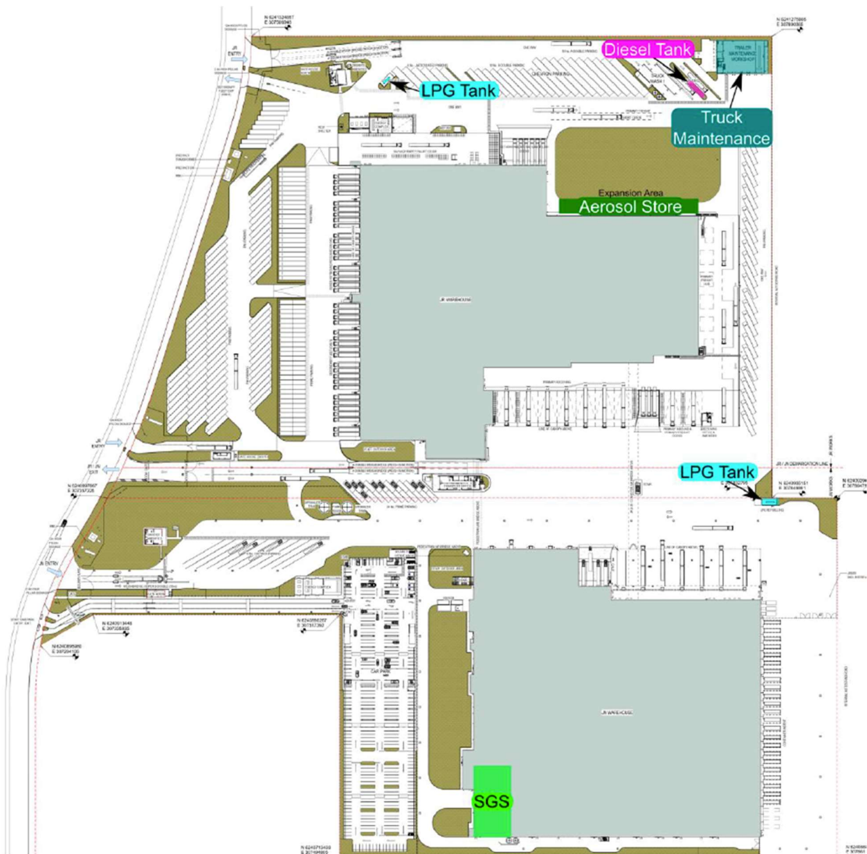
Figure 4-1 MORDC and MONDC Warehouses site layout with dangerous goods storage locations (Woolworths Limited – Final Hazard Analysis, Riskcon, 19 November 2021)
