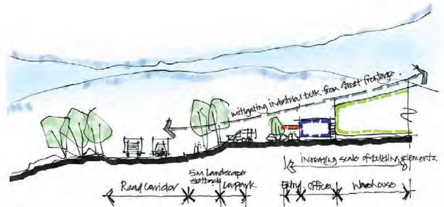
FIGURE 3.7 - Preliminary sketch displaying building setback strategy to mitigate the bulk form of industrial buildings at the street frontage.
