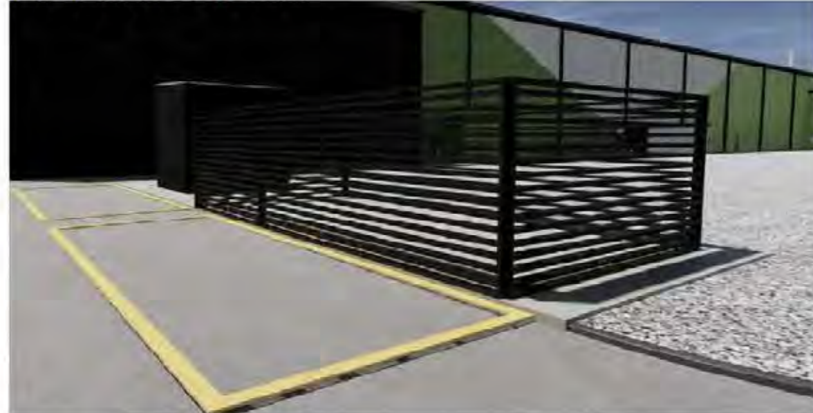
LOUVRE SCREENS: 1,800mm-2100mm HIGH, TYPICALLY POWDERCOAT FINISH COLOUR: MID GREY
