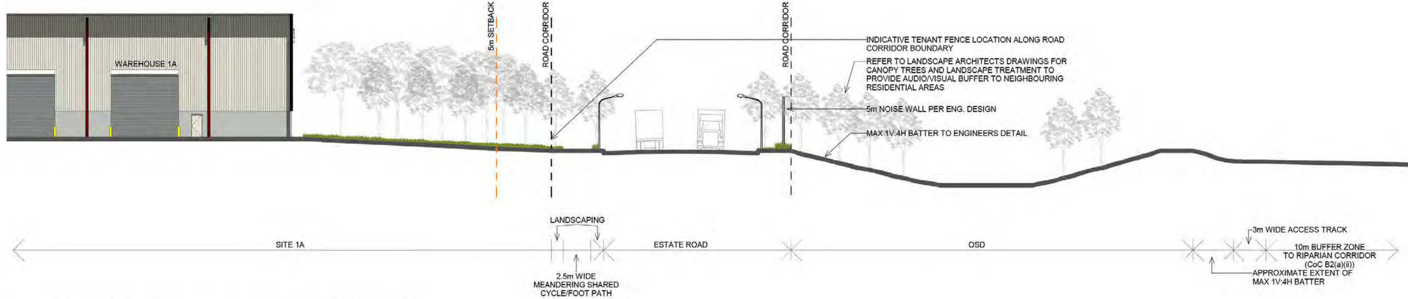
1 ROAD SECTION 01 - WAREHOUSE TO OSD 1 : 200
