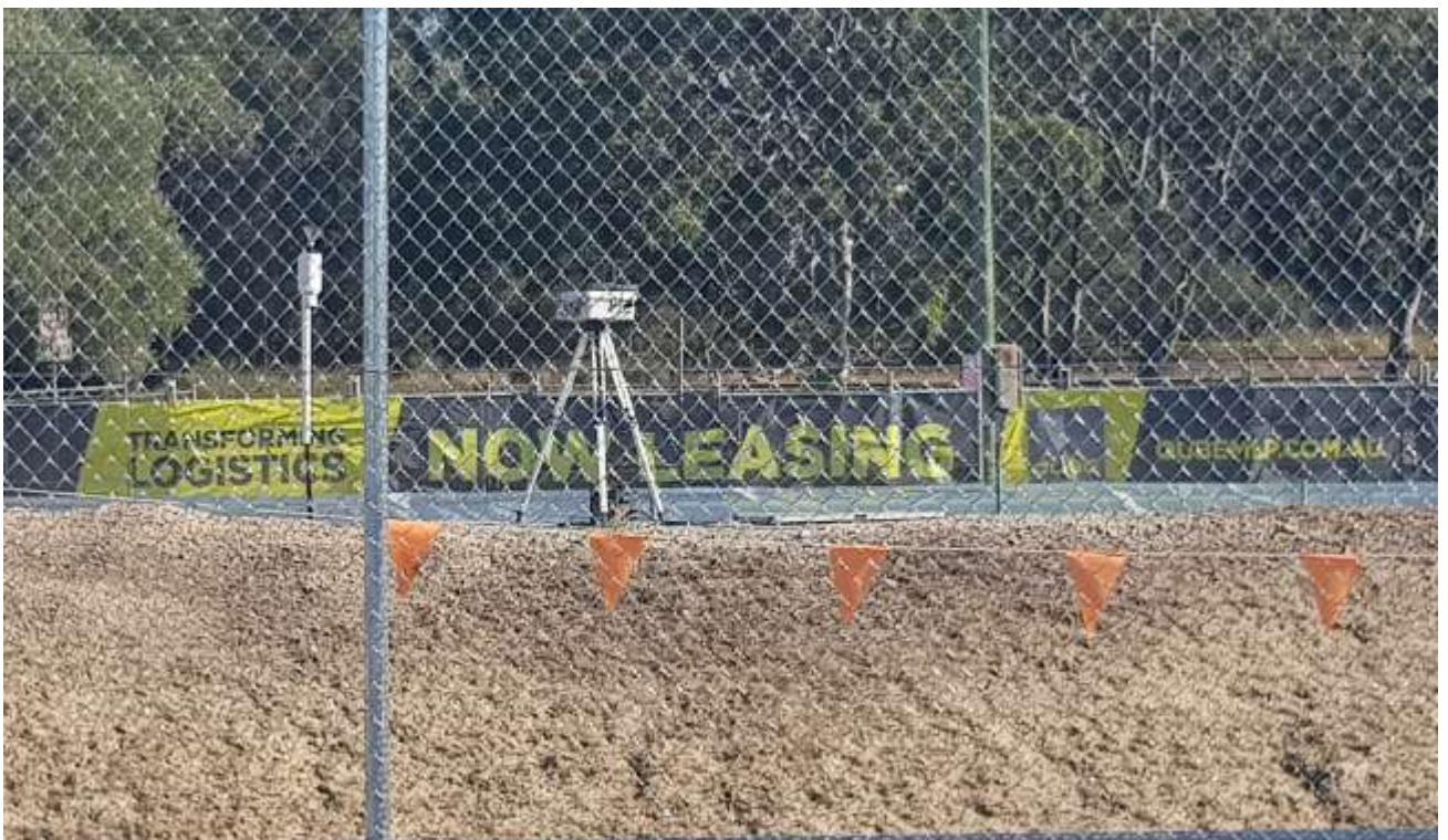
Photo 8: boundary dust monitoring
