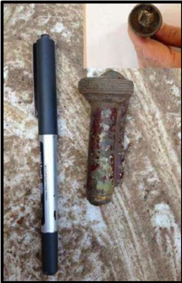
Figure 4: Mills 36 Hand Grenade Detonator Assembly
