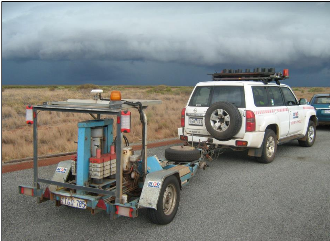
Figure 2.1: Falling weight deflectometer (FWD)
