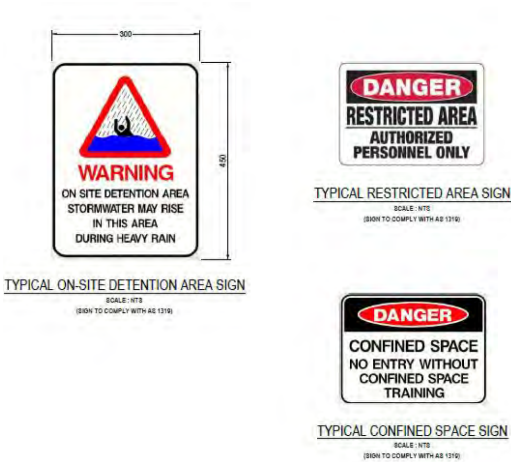
Figure 5-1: Typical OSD warning and danger signage.
