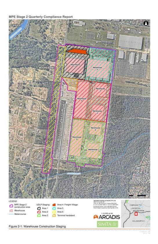
Figure 1-2 Warehouse construction staging
