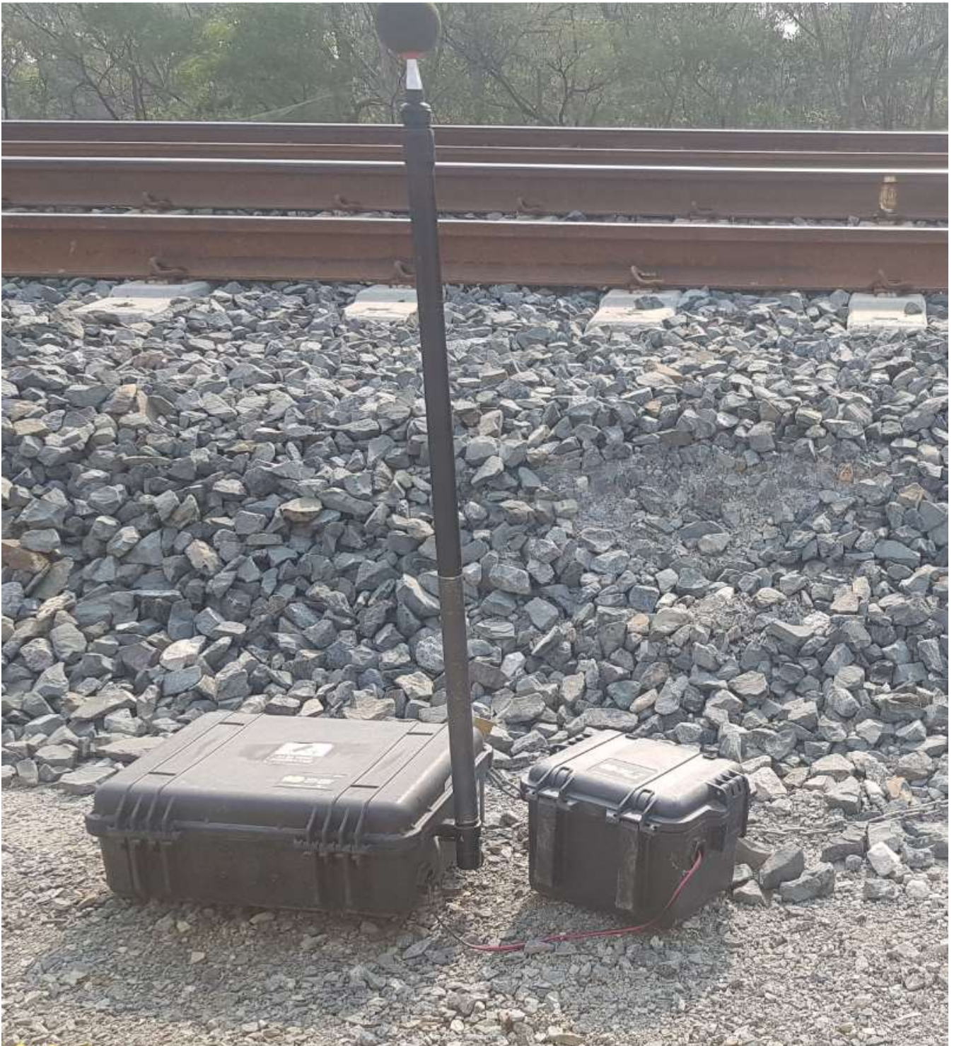
Figure 4: Angle of attack noise monitoring station (part of the plan prepared under CoC G7 and G7A).
