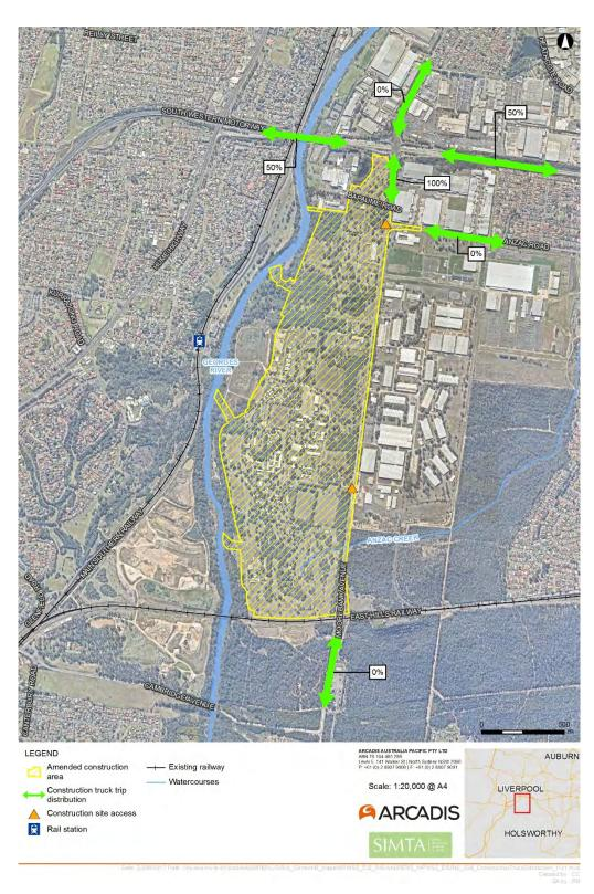
**Figure 5-2 Construction Truck Trip Distribution**
