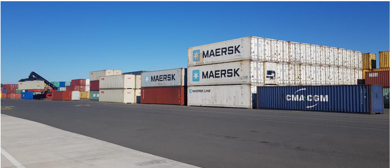
Photo 4: Reach Stacker crane in operation, with Container Noise Barrier in place.
