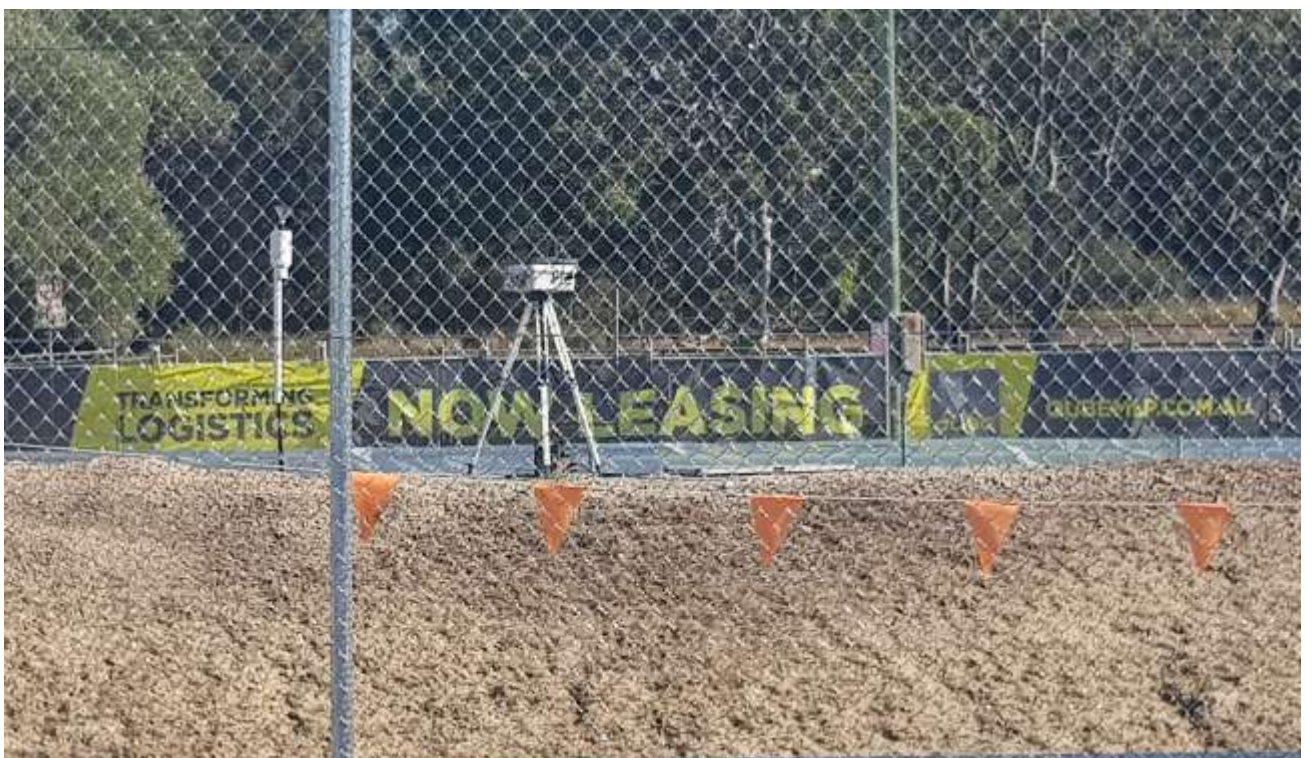
Photo 19: Boundary dust monitoring
