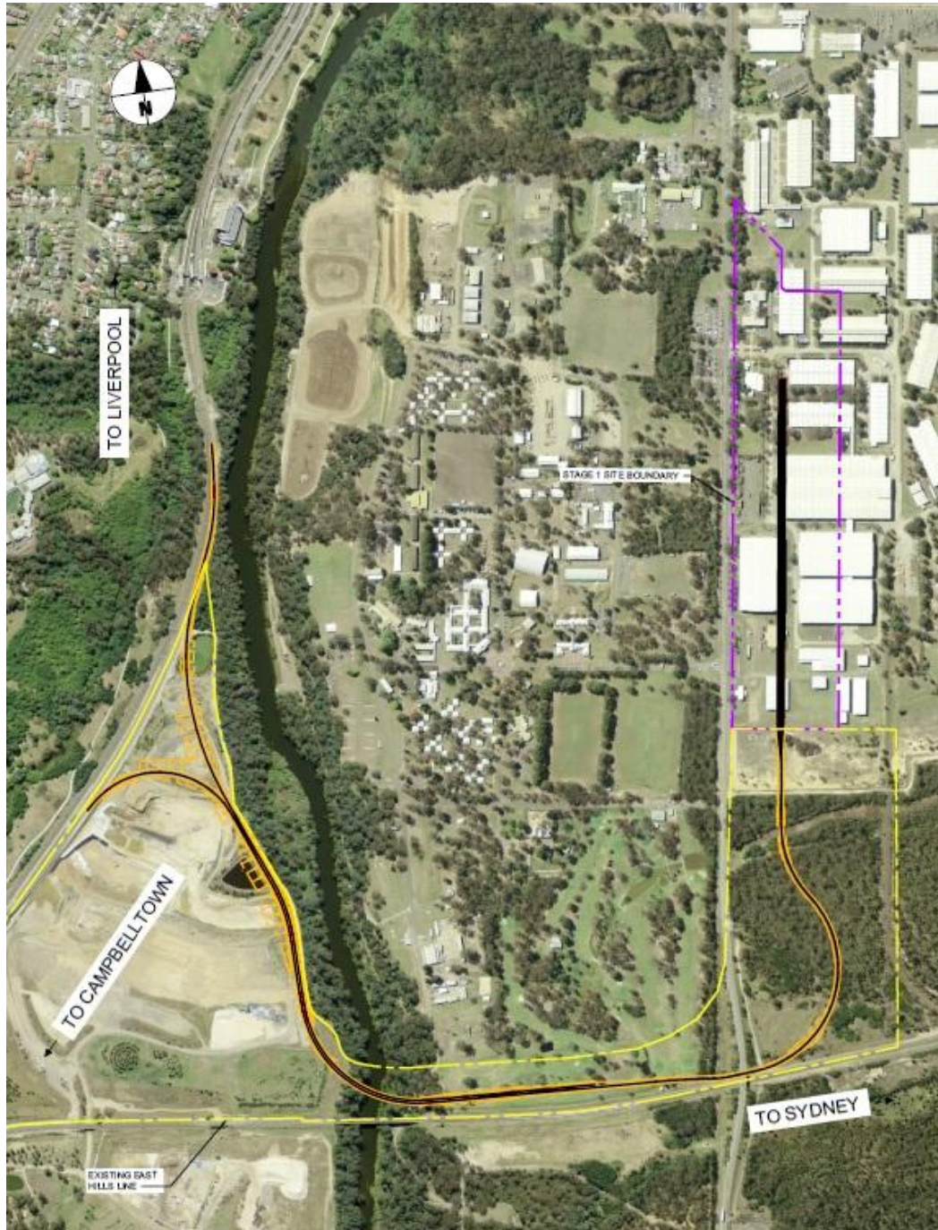
Figure 2 Moorebank Stage 1 Rail Link – General Arrangement
