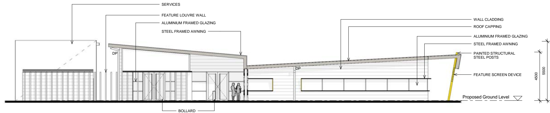
1 OFFICE NORTH ELEVATION A4200 1:100
