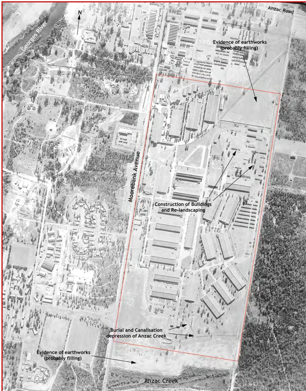
Figure A3: Aerial photograph of the study area in 1961. By this time the base's roads are formalised and re-landscaping is well established. Further earthworks, most likely the introduction of fill, have occurred in the southern and northeastern quadrant of the study area. The water depression of Anzac Creek within the study area has now been canalised (Source: Lands and Property Management Authority).
