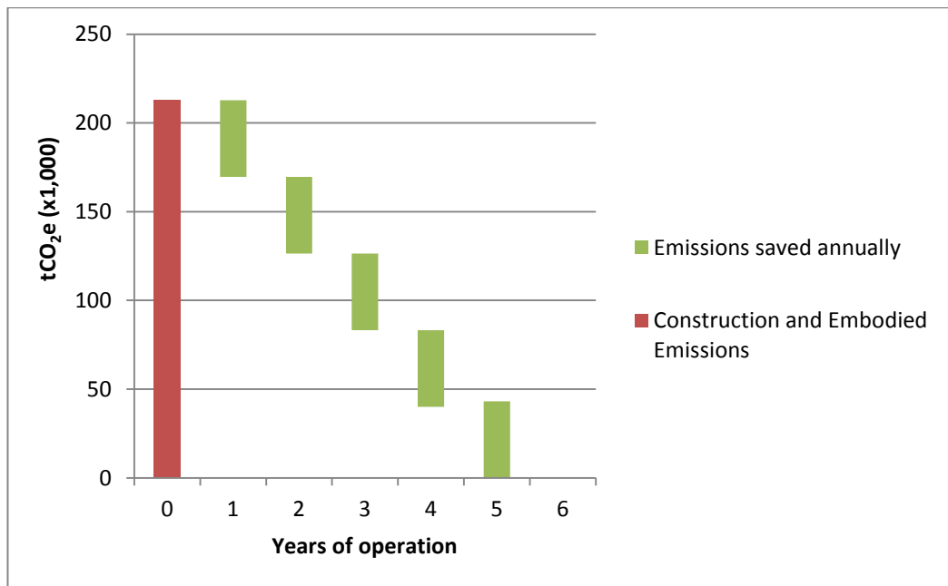
Figure 26: Annual emissions savings from operation of the SIMTA proposal equalising construction and embodied emissions in approximately 6 years of operation compared to the alternative scenario.
