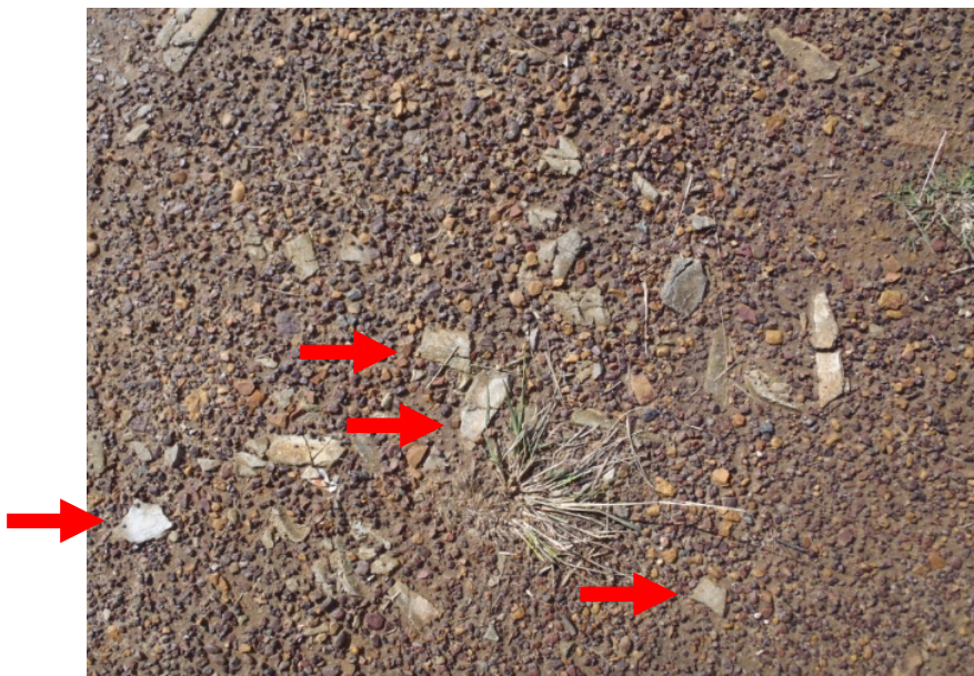
Plate 1: Potential ACM materials identified west of the existing rail spur
