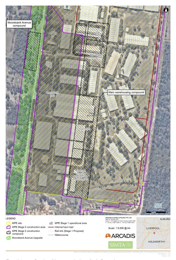
Figure 3-1 Overview of the construction layout for the Proposal
