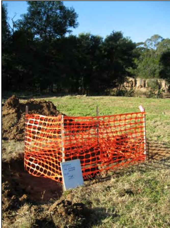
Figure 4.5 Test Pit 29 located on lower recent sandy alluvial deposits on western bank with higher level older regolith on eastern bank in background
