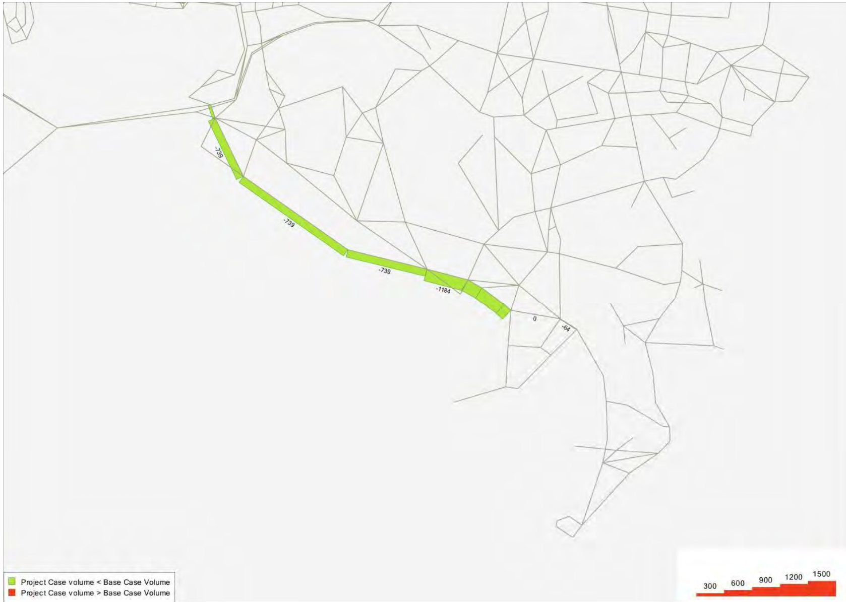
Figure D1.5 Change in articulated vehicle flows to/from Port Botany and Moorebank on Foreshore Road/Botany Road between Southern Cross Road and Bumborah Point Road
