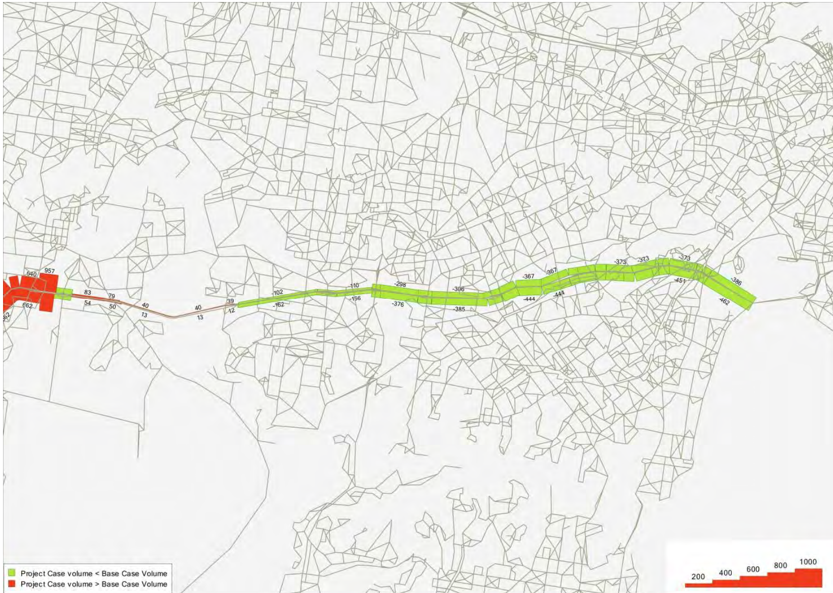
Figure D1.1 Change in articulated vehicle flows to/from Port Botany and Moorebank on the M5 between Sydney Airport and Hume Highway
